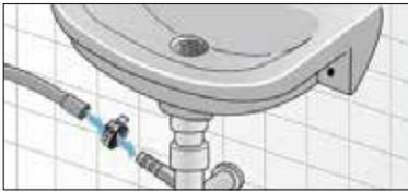
Secure the drain hose to the sink siphon using a  $\varnothing 0.9-1.6$  in. (20-44 mm) hose clip (available from a hardware store).
